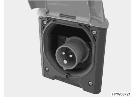
Fig. 117 230 V connection on the vehicle (CEE socket outlet)
