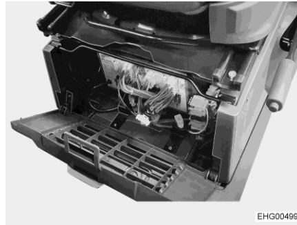
Fig. 112 Transformer/rectifier position (Stellantis)
