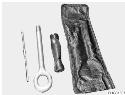
Fig. 184 Towing eye and screwdriver (Stellantis-based vehicle)
