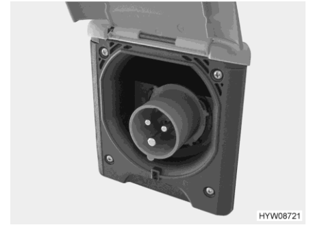
Fig. 87 230 V connection on the vehicle (CEE socket outlet)
