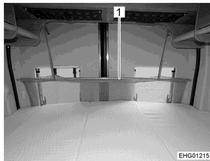
Fig. 58 Fall out protection (longitudinal rear bed)
